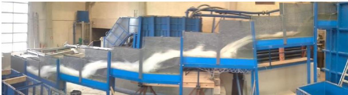
**Figure 8. Hydraulic modelisation on the reoxygenation sill ( $Q = 50 \text{ m}^3/\text{s}$ )**
